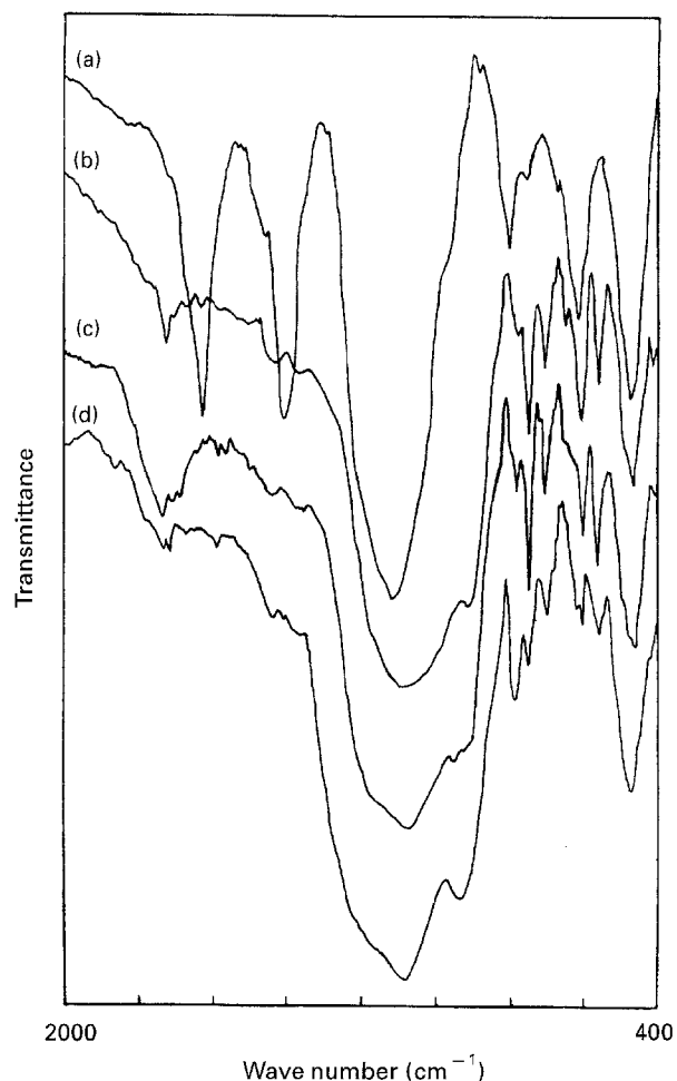
Figure 4 Infrared spectra of cordierite colloidal gel heated at several temperatures: (a) 40 °C for 60 h, (b) 900 °C for 9 h, (c) 1000 °C for 9 h, (d) 1100 °C for 9 h.
